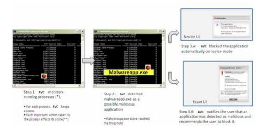
Applications and process are continuously monitored for as long as they are active for signs of suspicious, malware-like activity, including:
